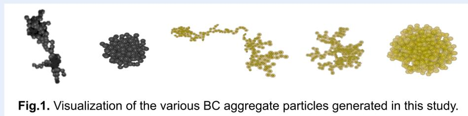
Fig.1. Visualization of the various BC aggregate particles generated in this study.
